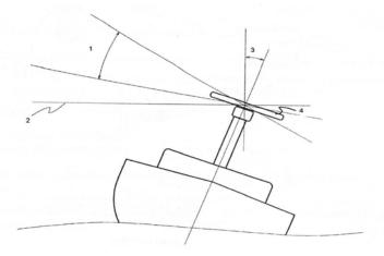
In this case, you're recommended to install the scanner on a gimbal mounting so that it can operate effectively in a heavy swell or when the yacht is heeled over.
